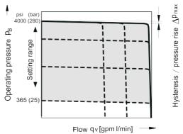
In order to prevent damage to the pump and the system, this setting range is the permissible setting range and must not be exceeded. The range of possible settings at the valve are greater.
