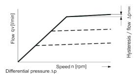
Standard setting: 200 to 320 psi (14 to 22 bar). If another setting is required, please state in clear text. Relieving the load on port X to the reservoir results in a zero stroke ("standby") pressure which lies about 15 to 30 psi (1 to 2 bar) higher than the differential pressure  $\Delta p$ . System influences are not taken into account.
